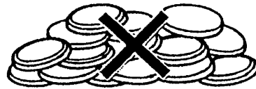
Example of stacked and jumbled batteries
