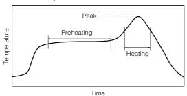
For soldering (Example : Sn/Pb)
