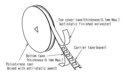
Fig. 2 Embossed Taping
