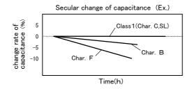
(5) When measuring the initial capacitance, perform the heat treatment at a temperature of  $150+0/-10^{\circ}$ C for one hour, leave it in a normal temperature and humidity environment for 48  $\pm$  4 hours, and measure the initial value.
