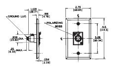
Wall plate with one B3M or B4M male receptacle mounted (in "D"-shaped hole to prevent turning) on standard single electrical outlet box. Cover mounting screws included.
