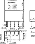
0.8±0.1 0.6±0. (1) : Input (2)(3)(4) : Ground (5) : Output (in mm)
