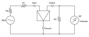
Rg+R1 =R2 : Input/Output Impedance
