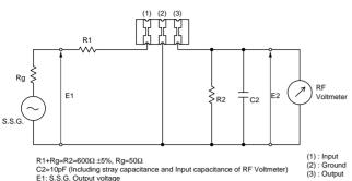
R1+Rg=R2=6000  $\pm 5\%$ , Rg=500 C2=10pF (Including stray capacitance and Input capacitance of RF Voltmeter) E1: S.S.G. Output voltage
