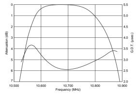
SFELF10M7GA00-B0 6.0 0 5.5 5.0 2 Attenuation (dB) 4.5 (: 4.5 Shi 3 4.0 D 3.5 5 3.0 6 7 2.5 10.700 Frequency (MHz) 10.500 10.600 10.800 10.900
