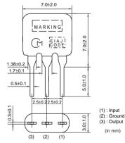
Spurious Attenuation Spurious Attenuation 3dB Bandwidth Center Nominal Center Input/Output Attenuation Insertion Loss Part Number Frequency (fo) (MHz) Frequency (fn) (MHz) Impedance (ohm) (kHz) (dB) (1) (dB) (kHz) (2) SFVLF10M7MF00-B0 10,700 fn±13 min 135 max. 5.0 +2.0dB 35 min. 330 fn±25 min. SFVLF10M7LF00-B0 \_ 10.700 5.5 ±2.5dB 30 min. 330 \_ 10.700 SFKLF10M7NL00-B0 20 min. 95 max. 6.0 max. 24 min. 600 ±15kHz SFELF10M7LFTA-B0 10.700 fn±25 min. 280 max. 7.0 ±2.0dB 30 min. 330
