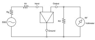
Rg+R1 =R2 : Input/Output Impedance
