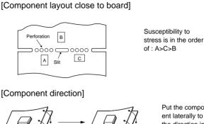
Put the component laterally to the direction in which stress acts.
