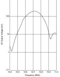
CDSCB10M7GA113-R0 1000 100 AF C 100 10 AF Output Voltage (mV) F.H.D. (%) Dis 10 0.1  $\begin{array}{l} \text{Input} = 100 \text{dB} \mu \\ \text{fdev.} = \pm 75 \text{kHz} \\ \text{fmod.} = 1 \text{kHz} \\ \text{Vcc} = 1.2 \text{V} \end{array}$ 10.3 10.4 10.5 10.6 10.7 10.8 10.9 11.0 11.1 Frequency (MHz)
