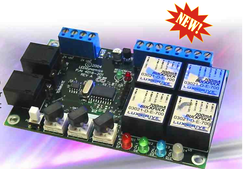
The 4016 QuadPuck LED Driver Interface with (4) 3021-D-E-0700 BuckPuck Drivers.
