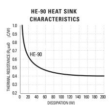
The HE-90 heat sink offers excellent thermal manage ment for up to three Series 1 type package SSRÕs or a single three phase SSR (Model 53TP). All mount ing holes are predrilled & tapped and are user configurable depending on the specific application.
