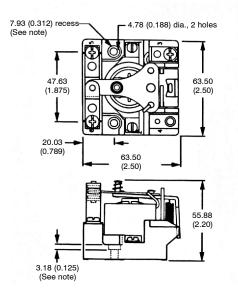
Note: Recess for screw mounting on units with 300-600 VAC coils
