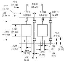
37D633 will mount eight 27E488 sockets in one length of aluminum strip measuring 10.97" x 2.25" x .062". (278.64 x 57.15 x 1.57)
