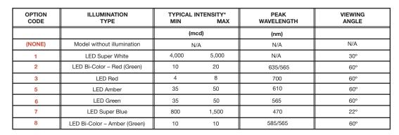
\*LED FORWARD CURRENT: 20 mA LED FORWARD VOLTAGE: 2.0 V TYP. LED REVERSE VOLTAGE: 5.0 V MAX
