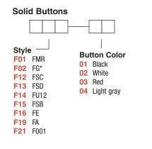
\*Button options for central mounting configurations, use 'FG' for central mount with chrome dress nut, use 'FA200' for central mount with black dress nut.
