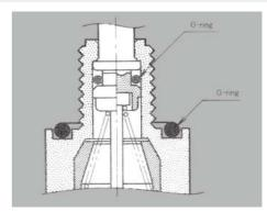
The splash proof push button switch is a panel seal switch to seal against ingress of moisture, etc. However, it cannot be used in water.
