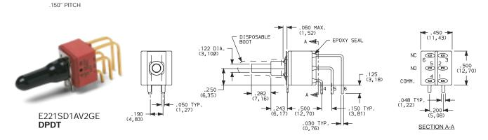
AV3 VERTICAL RIGHT ANGLE, SNAP-IN, PC THRU-HOLE, .150" PITCH
