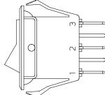
NOTE: Orientation of actuator marking and terminals. Shown in Pos. 1
