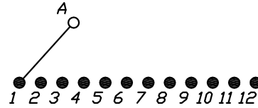
CONTACT CONFIGURATION Timing: SHORTING
