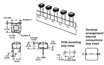
**Note:** The tape is random between surface A and surface B. Unit: mm (inch)
