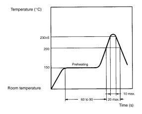
**Note:** The above curve is given on condition that the thickness of the PCB is 1.6 mm.
