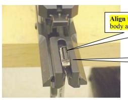
Align the orientation of the connector body and cover assembly.
