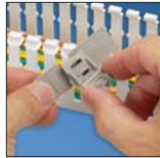
Labeling Outside Duct – Break off the last segment from wire retainer below (1.5" mark) and snap onto the back of the remaining segment. Install label and mount between fingers facing outward.
