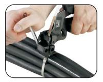
3. Maintain tension and rotate cut-off handle
