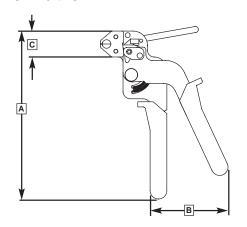
Overall length A = 8.5" (216 mm) Open handle span B = 4.0" (102 mm) Height of head C = 1.3" (32 mm)Weight 19 oz. (539 g)
