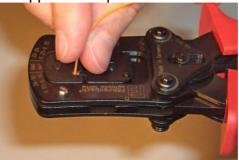
Keep the wire fixed in position and activate the levers till they reach the end
