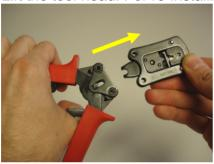
After a proper installation of the tool head, you can lock them by pushing the two
