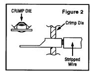
With the handles in the open position, depress die release and rotate die to desired pocket. The pocket will lock in place when an audible "click" is heard (Die index number and color appear to the left of corresponding pocket).
