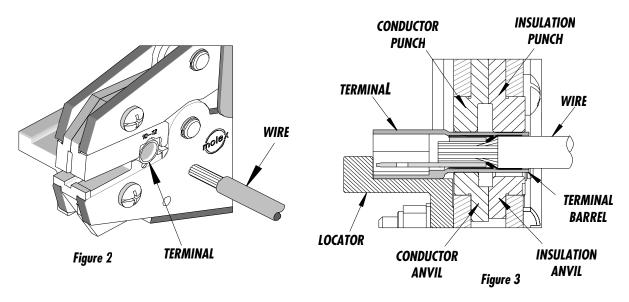
Note: Whenever crimping without the locator, make sure the seam of the terminal is oriented up or down in the tool if using unbrazed product, as this will provide higher pull force values.
