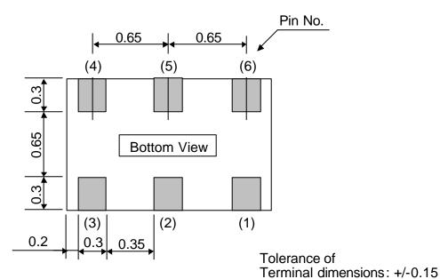
[Recommended PCB pad dimensions] Unit: mm
